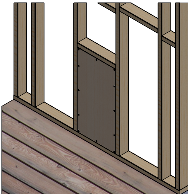
3. 18mm Plywood panel is added as support for the wall mount.
