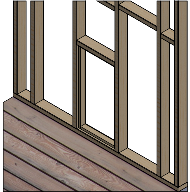
2. An extra noggin and battens are added to support a plywood panel.
