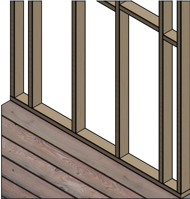
1. A typical timber stud (partition) wall.
